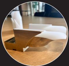
Two-Piece Wiper Dies are great for more difficult applications when additional support is required, such as 1D bending.
